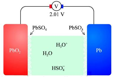
The theoretical capacity and specific power of a battery are rather easily calculated when simplifying assumptions are made. For example, in a fully charged lead-acid cell (diagramed and discussed on pages 56–57), 0.239 kg of PbO<sub>2</sub> at the positive and 0.207 kg of Pb at the negative (one mole of each) would theoretically require only 0.385 liters (weighing 0.499 kg) of 5.2 molar aqueous sulfuric acid to permit the cell reaction
