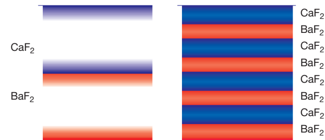
Figure 4 Comparison of conductivity profiles in the semi-infinite space-charge and mesoscale situations. The concentration or (parallel) conductivity profiles are sketched for the semi-infinite space-charge situation (period > 8\lambda , left), and for the mesoscale situation (period < 8\lambda , right) in which the space-charge regions overlap and bulk values are exceeded even in the centres of the individual layers.
