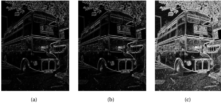
Figure 14.11. Computing the gradient. The image obtained from the computed gradient is shown in (a) and in (b) the numbers have been normalised. In (c) the contrast has been enhanced with a logarithmic function.
