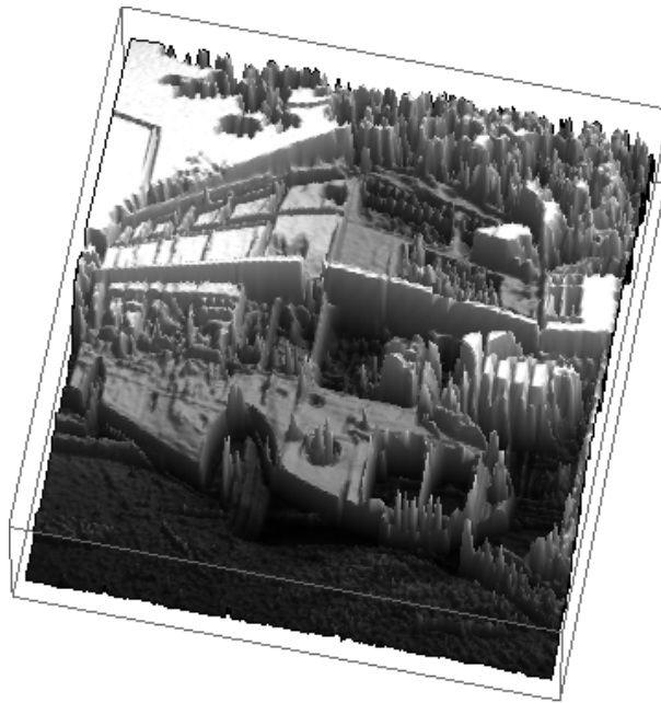
Figure 14.3. The grey-level image in figure 14.1 plotted as a surface. The height above the (x, y) -plane is given by the intensity value.
