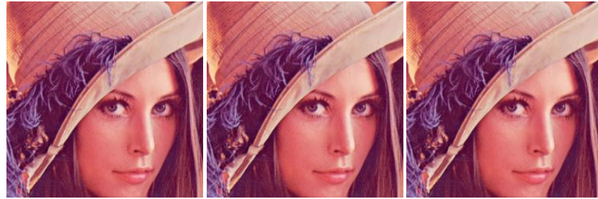
(a) Threshold 30. 91.4% of the DFT-values were neglected (b) Threshold 50. 95.3% of the DFT-values were neglected (c) Threshold 100. 97.7% of the DFT-values were neglected
