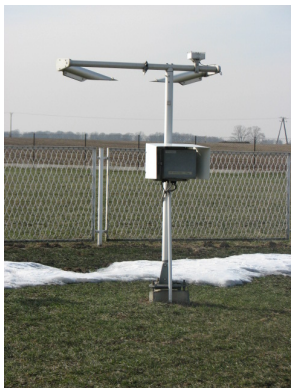
Figure: Vaisala FD12P, All in one Weather Sensor.
