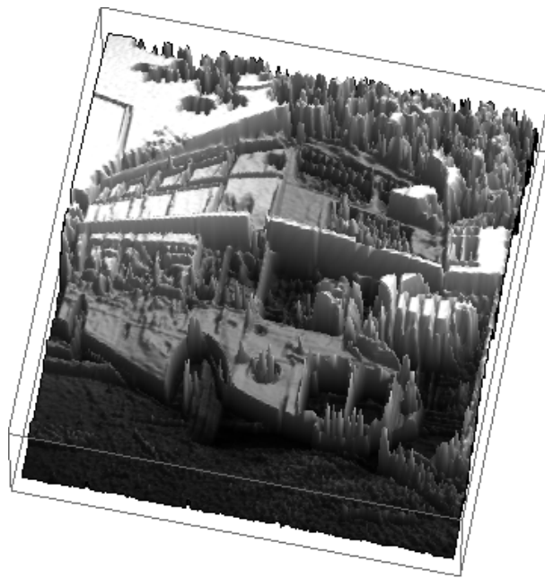
Figure 6.3: The grey-level image in figure 6.1 plotted as a surface. The height above the (x, y) -plane is given by the intensity value.
