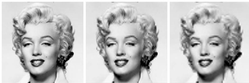
(a) Resulting image after also neglecting detail in W_2^{(1,1)} , as illustrated in Figure 8.10(a). (b) Resulting image after also neglecting detail in W_2^{(1,0)} , as illustrated in Figure 8.10(b). (c) Resulting image after also neglecting detail in W_2^{(0,1)} , as illustrated in Figure 8.10(c).
