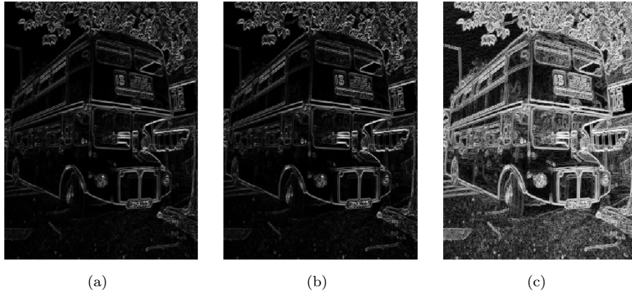
Figure 6.11: Computing the gradient. The image obtained from the computed gradient is shown in (a) and in (b) the numbers have been normalised. In (c) the contrast has been enhanced with a logarithmic function.
