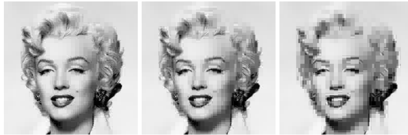
(a) Threshold 30. 91.3% of the DFT-values were neglected (b) Threshold 50. 94.9% of the DFT-values were neglected (c) Threshold 100. 97.4% of the DFT-values were neglected
